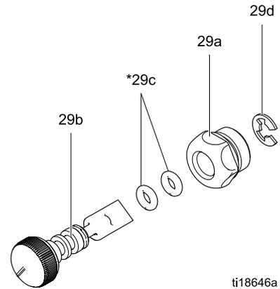
Figure 49 雾化空气节流阀
